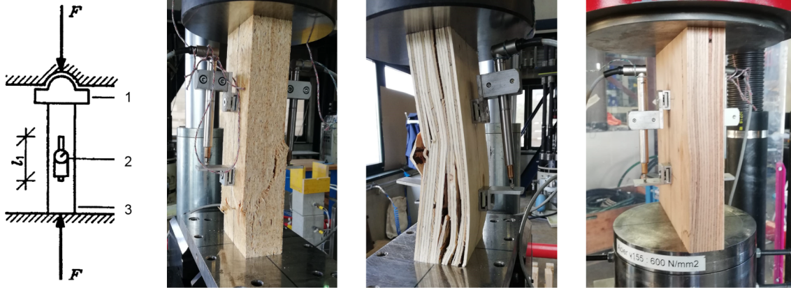
Fig. B.13. Compression setup: (a) EN789 [30] (1) Spherical seated (2) Transducer (3) Test piece/ (b) OSB specimen/ (c) Spruce LVL specimen/ (d) beech LVL specimen.
