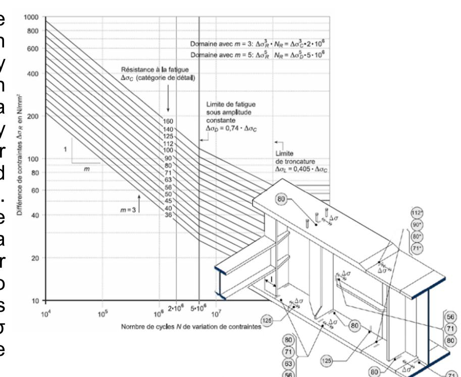
The lambda method is a fatigue verification that has been developed to simplify the cumulative damage method, introducing lambda correction factor that correlates this last to the Fatigue Load Model 3, a simplified model easy to calculate for the engineers.  $\Lambda \sigma_{c}$
