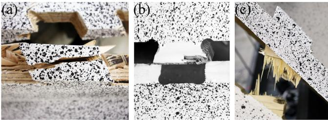
Figure 14: MTSJ failure modes; (a) open slot; (b) open slot ( $\theta_1 = 0^\circ$ ,  $\theta_2 = 27^\circ/0^\circ$ ,  $\theta_3 = 20^\circ$ ); (c) closed slot.
