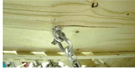
Figure 16: MTSJ with closed slots, replicate 3. Failure along the middle of the loaded plate bottom face.
