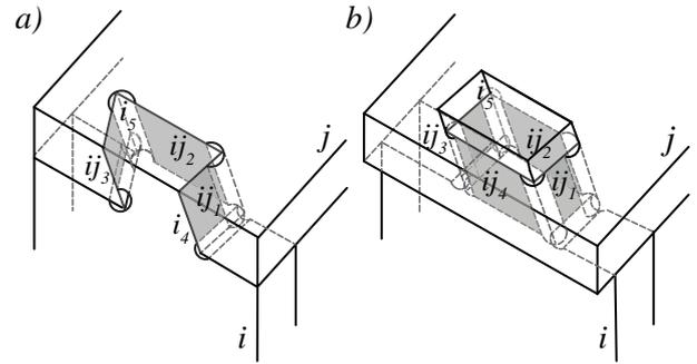
Figure 17: MTSJ contact faces pairs; (a) open slot; (b) closed slot.
