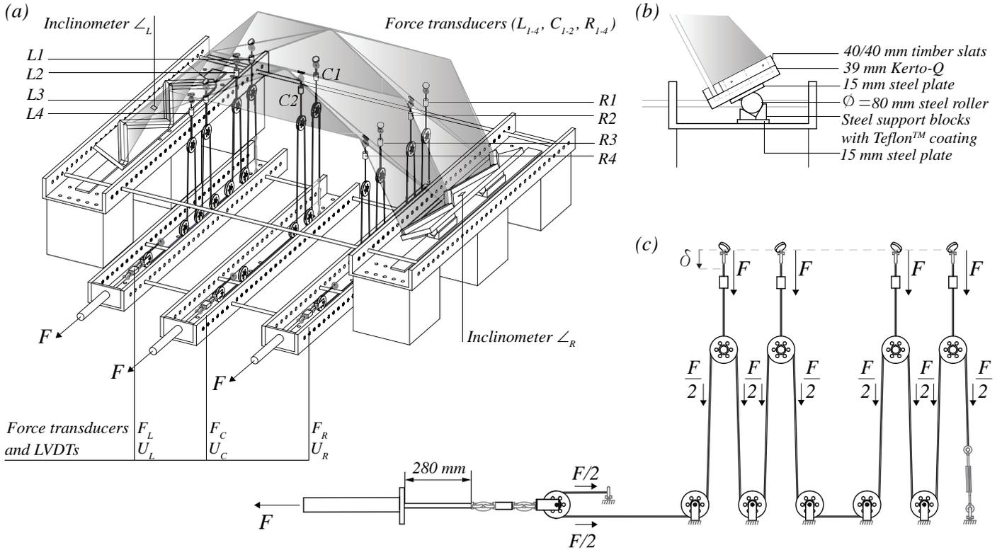
Figure 9: (a) Test setup with marked measurement instrumentation; (b) Side support detail; (c) Load application setup schematic.
