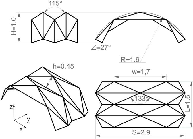
Figure 2: Large scale structure geometry parameters
