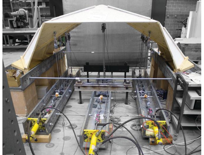
Figure 1: Test setup devised for approximating uniformly distributed surface load.
