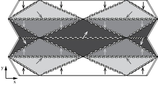
Figure 4: MTSJ plate insertion vectors and assembly sequence of the chosen folded form. Plate grayscale range illustrates the order of assembly, black represents the first and white the last plates to be put in position. Arrows display the insertion vectors.
