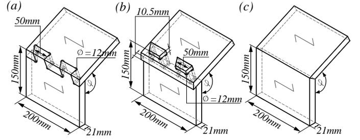
Figure 3: Test detail geometry parameters,  $\varphi = 115^\circ$ ; (a) MTSJ with open slots; (b) MTSJ with closed slots; (c) Miter joint.
