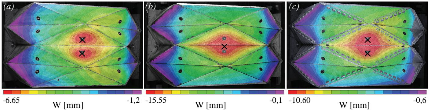
Figure 11: Displacement fields of each of the tested structure type unfavorable replicate, shown at the moment when the total load on the structure amounted to  $25kN$ ; (a) Adhesively joined structure, replicate 3; (b) MTSJ with open slots, replicate 3; (c) MTSJ with closed slots, replicate 3. Points at which the displacement data was extracted for each type are marked with  $\times$ , in case of (a) and (c) as the maximum displacement found around the loading ring.
