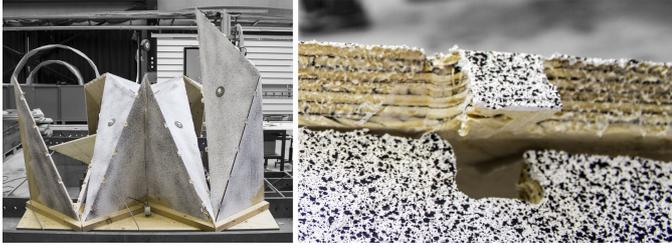
Figure 13: Loss of structural integrity in adhesively joined structures after point (D)(left) and detail of edge after failure (right); Replicate 3 is shown as a representative of all three tested replicates since they exhibited same type of final collapse.
