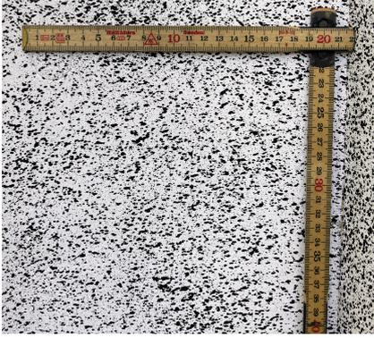
Figure B.21: Speckle pattern with speckle sizes between 1-5mm.
