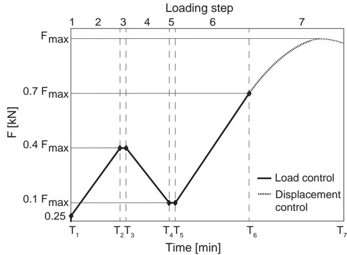
Figure B.22: Loading procedure.
