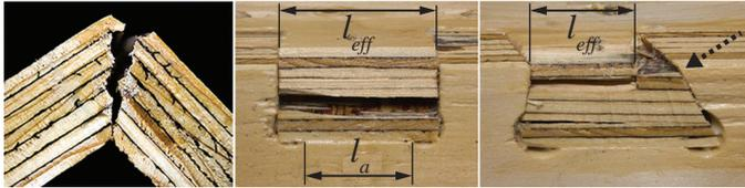
Figure 6: Failure of adhesively bonded connections; from left to right: miter joint, finger joint, MTSJ with open slots. In MTSJ with open slots dashed arrow points to the surface where additional compression occurs.
