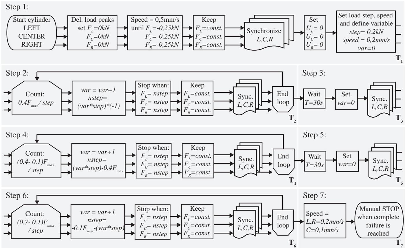
Figure B.23: Test loading process, separated according to the defined seven loading steps.
