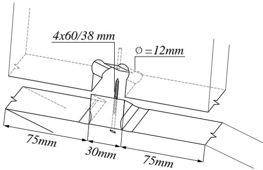
Figure 8: One-faced finger joint with a screw for applying pressure. Joint spacing along the edge was taken as 180 mm; in this figure pressure area of only one screwed joint is shown.
