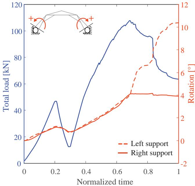
Figure 15: Total load and rotation of supports vs. normalized time shown on the example of MTSJ open slot replicate 3. Sudden increase in rotation of left support occurs at the moment of MTSJ failure at the left side connection between half and full-sized plate. Both MTSJ open and closed slot structure replicates experienced the same reaction, where the support side with rotation increase varied depending on the failure side.
