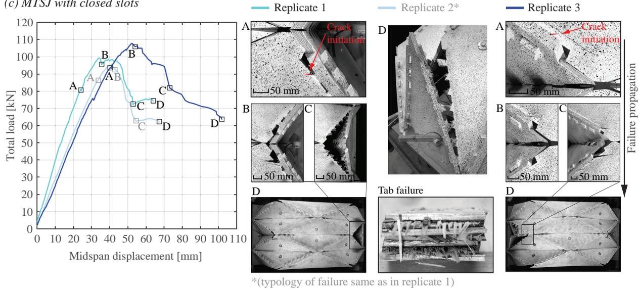
Figure 12: Individual total load vs. midspan displacement graphs and failure propagation for each of the tested structure type.
