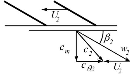
**Fig. 2 Velocity triangle at the runner exit**
