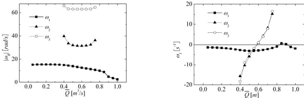
**Fig. 8** Effect of  $\bar{Q}$  to first 3 order frequencies at  $L_i = 50$  m, under  $a = 500$  m/s
